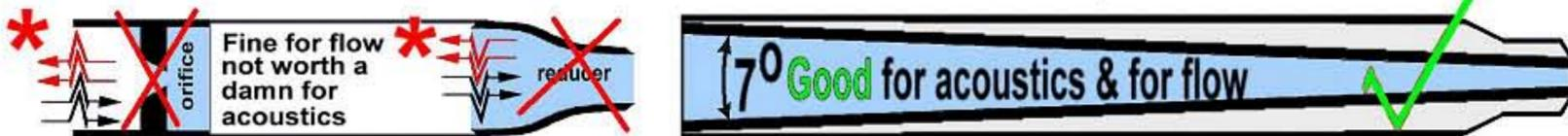
Nearly all of a pressure spike can be caused to go into a damper from a large diameter pipe by compressing it down a 7° taper. \* is "PULSE REFLECTION"
